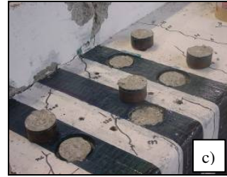
Fig. 7 - Pull-off tests: a) steel plates bonded to the CFRP; b) test; c) failure modes
