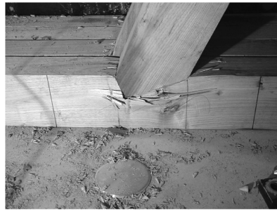
Figure 3. Typical experimental failure patterns: joint collapsed in compression, with uniform distribution of damage.
