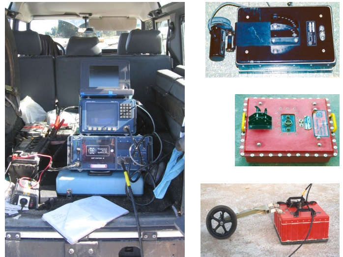
Figure 3 – Equipment: System SIR-10 – GSSI, and antennas of 900, 500 and 200 MHz.
