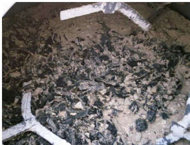
Fig.1 – Rubber particle during the mixture of concrete [25]
