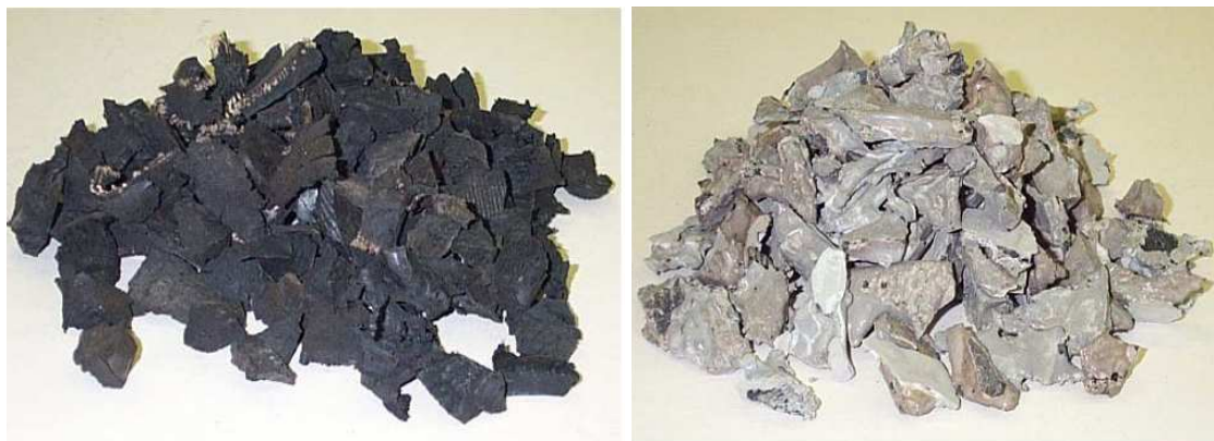
Fig.2 – 20 mm rubber aggregate particles: a) Plain; b) Coated with cement paste [5]
