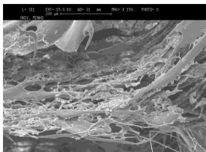
Fig. 3. Micrograph of a location in screw turn 7 showing the the morphology evolution from sheets to droplets (PA6/PP 80/20 wt.%).
