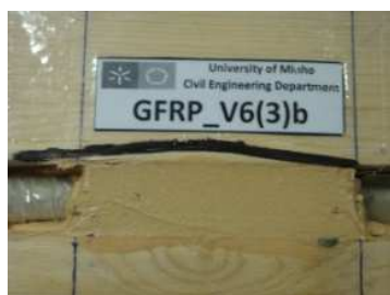
GS – Glulam shear failure
