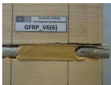
GAI – Glulam/adhesive interfacial sliding
