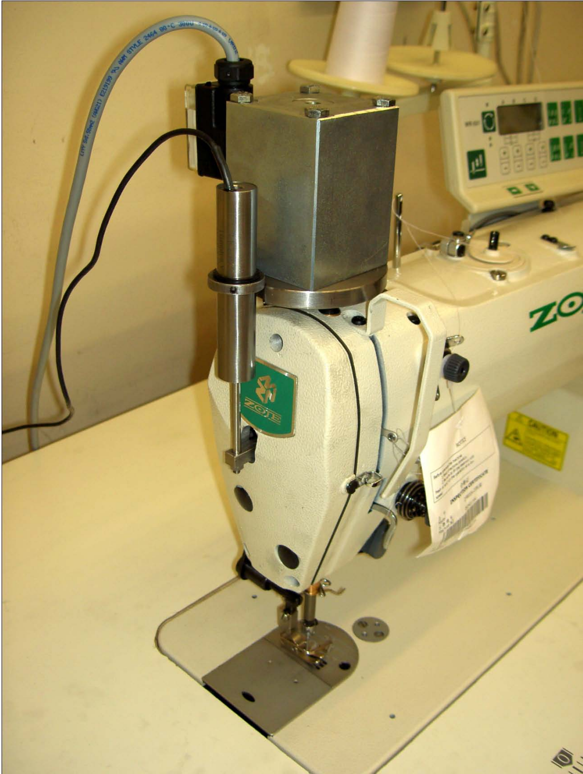
Figure 3. Hardware set-up of the controller.
