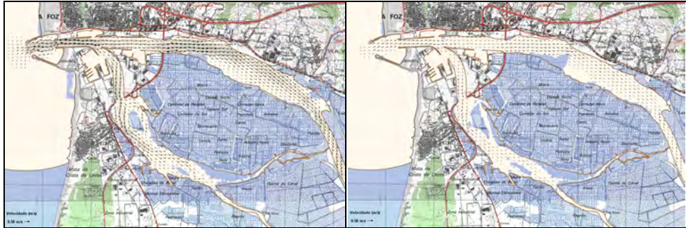
Fig. 16. Effect of tidal regime on ebbing maximum values of currents velocity magnitude (scenarios H2 and H3)
