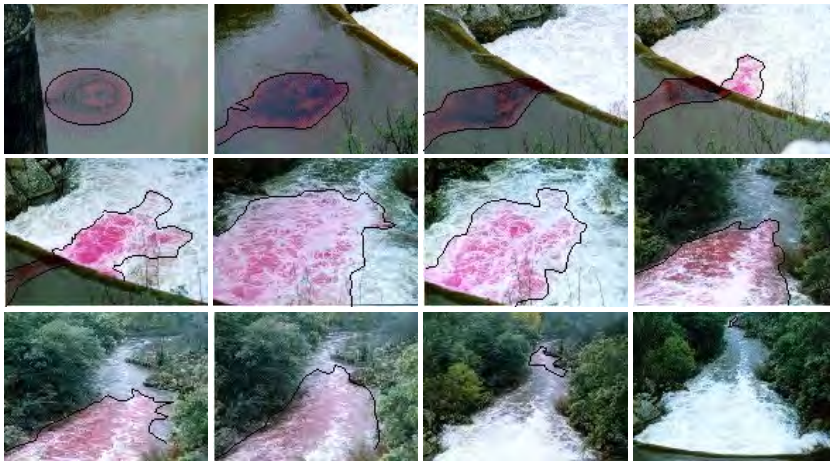
Fig. 11. Rhodamine spreading after their injection in a river Mondego reach
