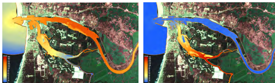
Fig. 22. Effect of Pranto river discharge on RT values distribution (scenarios RT1 and RT6)
