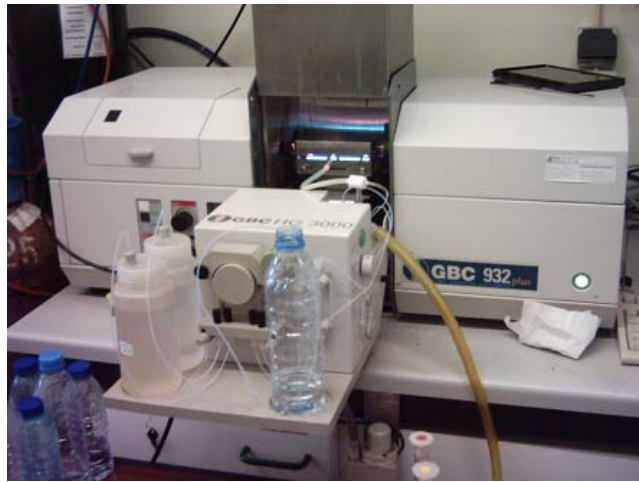
Figure 3 Samples analysis using the AAS technique with the hydride generation module
