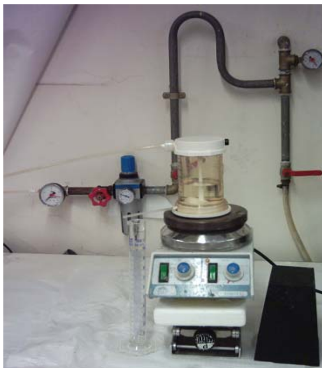
Figure 2 Laboratory installation used for membrane separation tests
