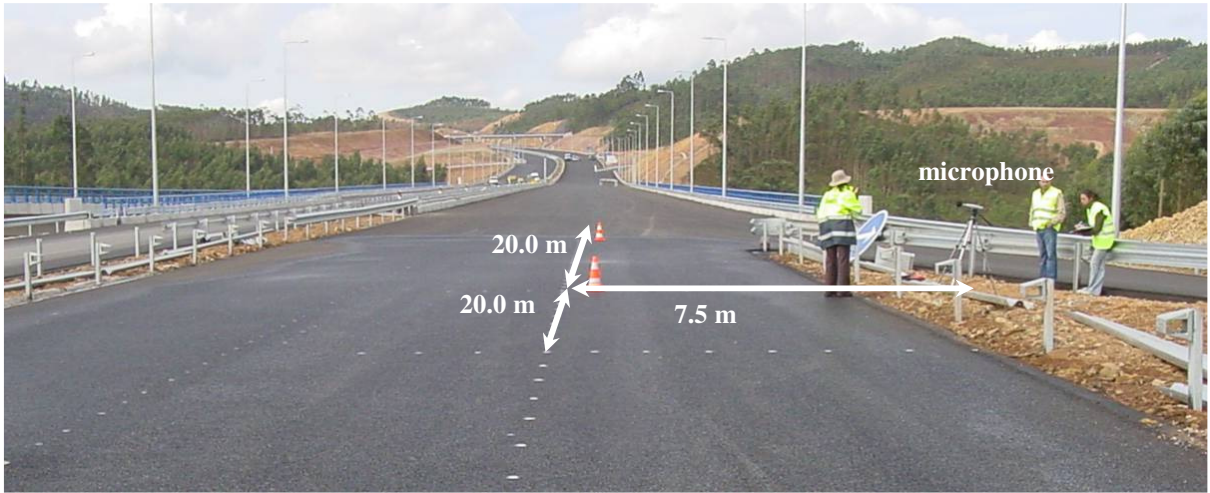
Figure 1 – Location of the sections and layout of the tests
