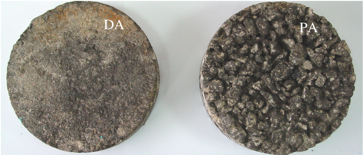
Figure 2 – Aspect of the wearing course (DA – Dense Asphalt, PA – Porous Asphalt)
