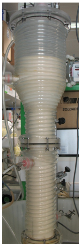
Figure 3.4 - Airlift bioreactor with biotransformation medium.
