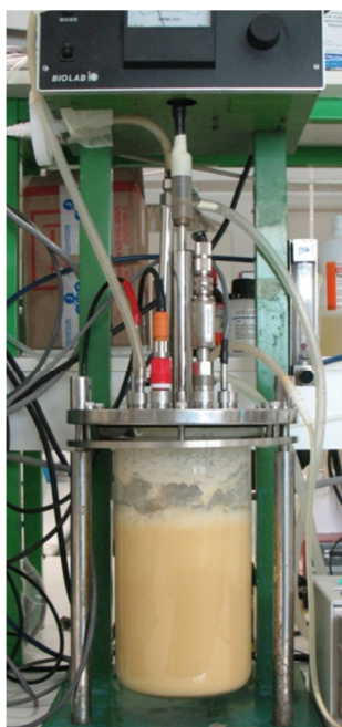
Figure 3.1 - BIOLAB bioreactor with biotransformation medium.
