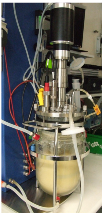
Figure 3.2 - RALF PLUS SOLO bioreactor with biotransformation medium.
