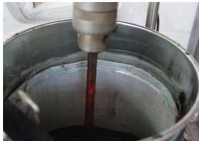
Figure 1. Production of the asphalt-rubber binder.
