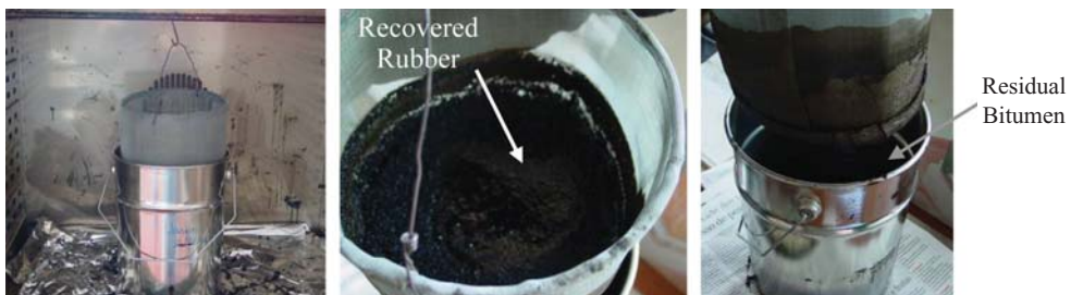
Figure 2. Separation of the AR binder in its constituents (residual bitumen and recovered rubber).
