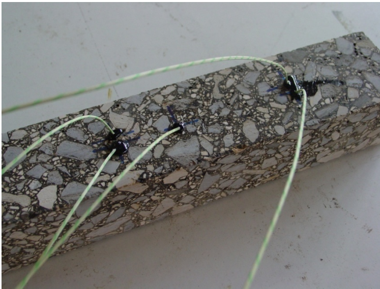
Figure 14. Test sample with thermocouples for temperature measurement
