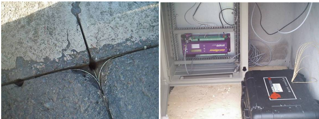
Figure 2. Pavement instrumentation and data acquisition
