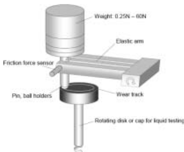
Figure 1 The pin-on-disk tribosystem (schematic arrangement)
