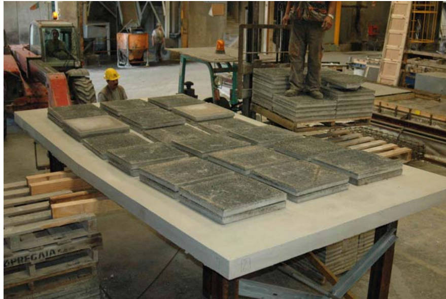
Fig. 12. Final view of the panel, loaded with 33 concrete plates.
