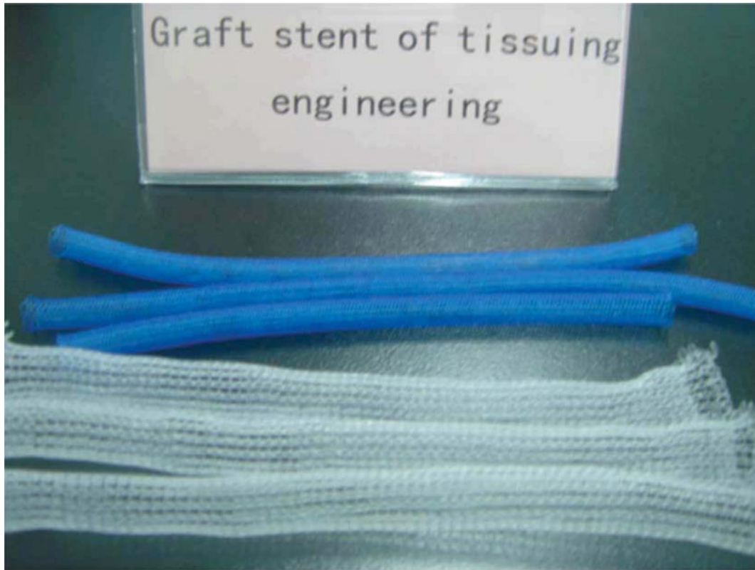
Figure 1. Samples manufactured (knitted in the foreground and braided in the back).
