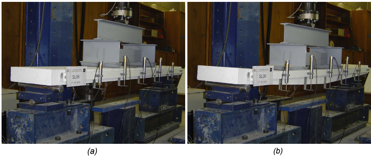
Figure 6.5 - Specimen SL2 before (a), and after having been tested (b).
