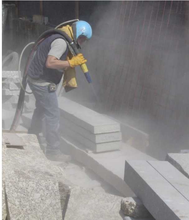
Figure 5.5 - Sandblasting the top surface specimen.
