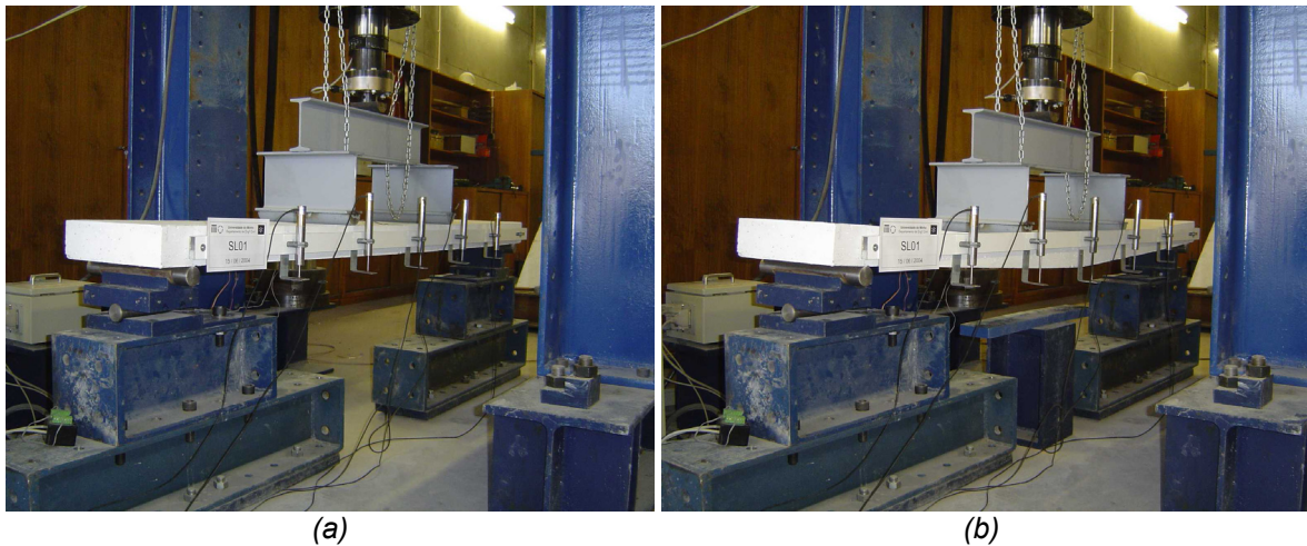
Figure 6.1 - Specimen SL1 before (a), and after having been tested (b).
