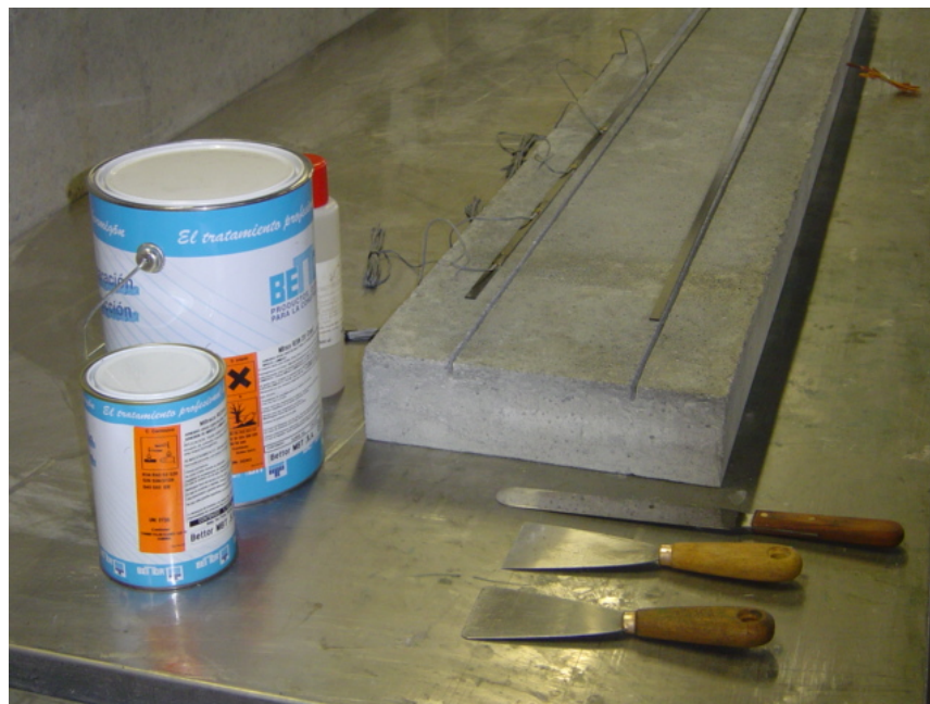
Figure 5.3 - A specimen before being strengthened; the adhesive compound recipients; the acetone bottle; the CFRP laminate strips; and the tools used to mix and to apply the epoxy adhesive into the slits.
