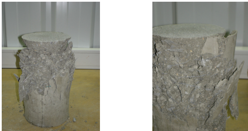
Figure 3.19: Typical failure mode of compression tests
