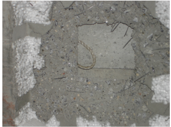
Figure 4.20: Failure surface in a punching test
