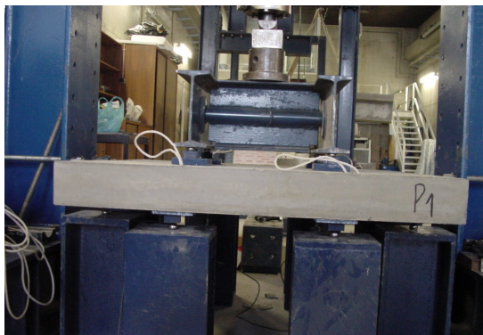
Figure 4.10: Panel prototype being tested in bending
