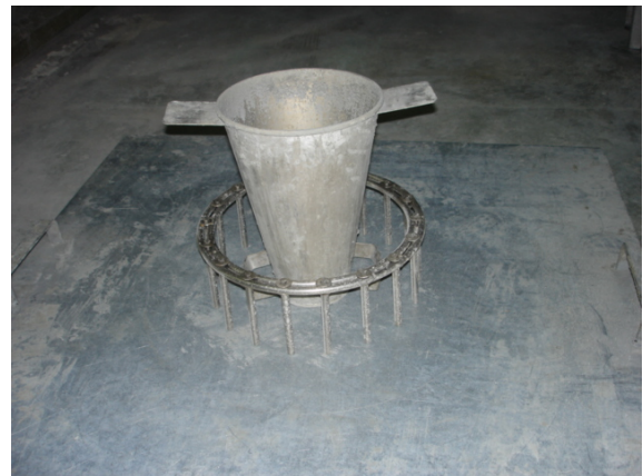
Figure 2.5: Combination of J-Ring with Abrams Cone
