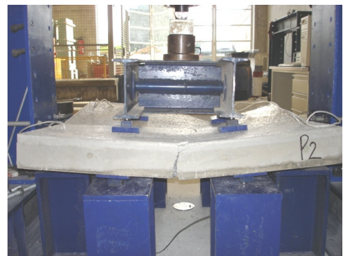
Figure 4.10: Panel prototype being tested in bending
