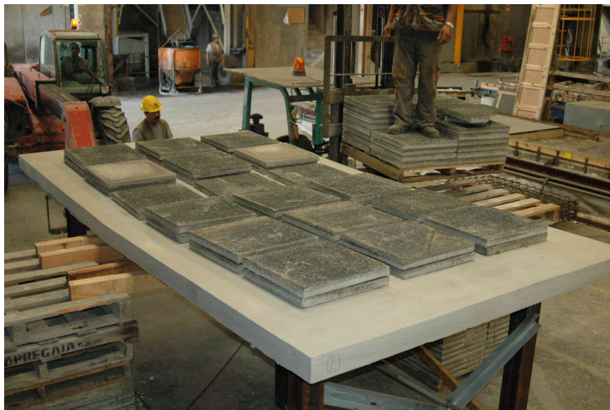
Figure 5.7: Final view of the panel, loaded with 33 concrete plates
