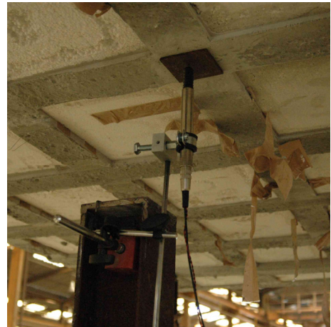
Figure 5.5: LVDT for measuring the panel deflection at its center
