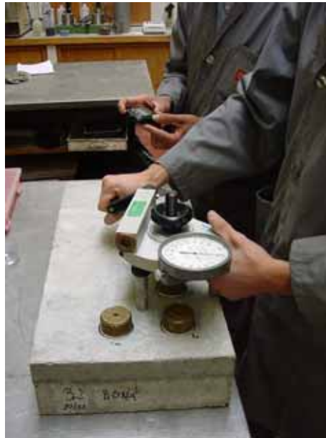
Figure 05 - Testing with Proceq DYNA Z15.
