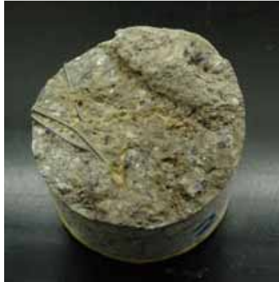
Figure 14 - Detail of the failure mode verified in the test 2 of the model B1C1P2.
