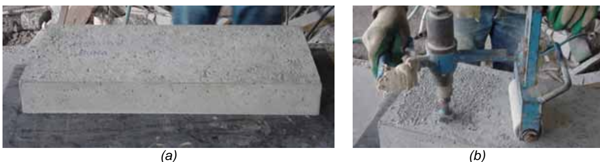
Figure 01 - The specimen surface before roughing (a) and the rough machine (b).
