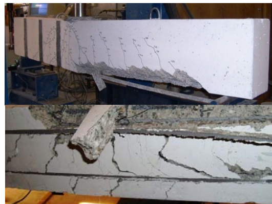
Fig. 6 Crack pattern of the lower face of VLM2 along the L_2 span, at the end of the test
