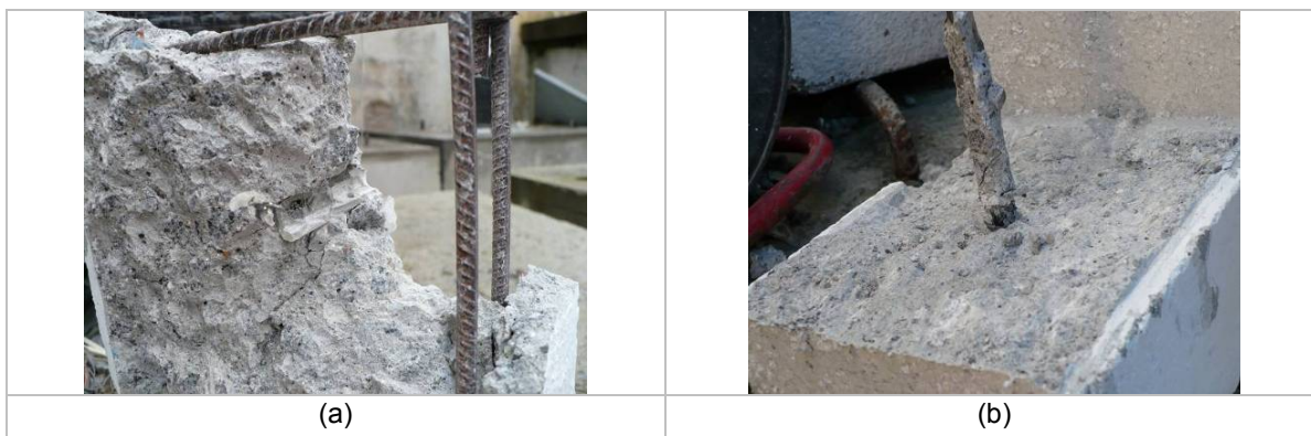
Figure 7: Failure modes: (a) CS1 and (b) CS2 specimens
