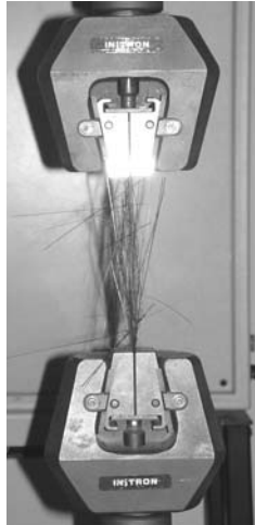
Figure 6. Typical failure mode in the uniaxial tensile tests.
