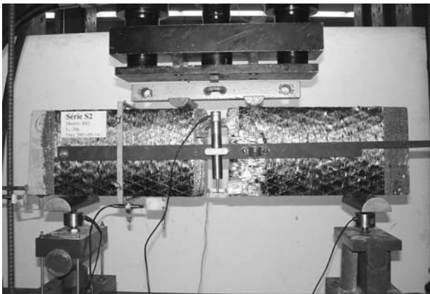
Figure 13. Carbon sheets to increase the shear strength of the specimen.
