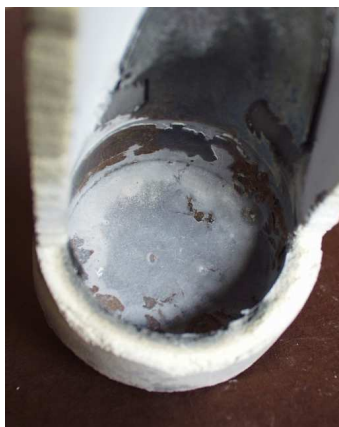
Figure 7. Portion of a Y_2O_3 partially stabilized ZrO_2 crucible with inside Y_2O_3 layer, after melting a Ti-48Al alloy. The Y_2O_3 film is still visible at the inside crucible wall, and no cracks are detected.
