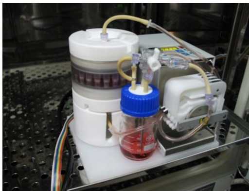
Figure 5.1 – Multichamber flow perfusion bioreactor (PT Patent n° 104155; European patent pending [24]) assembled and the culture system inside the incubator.
