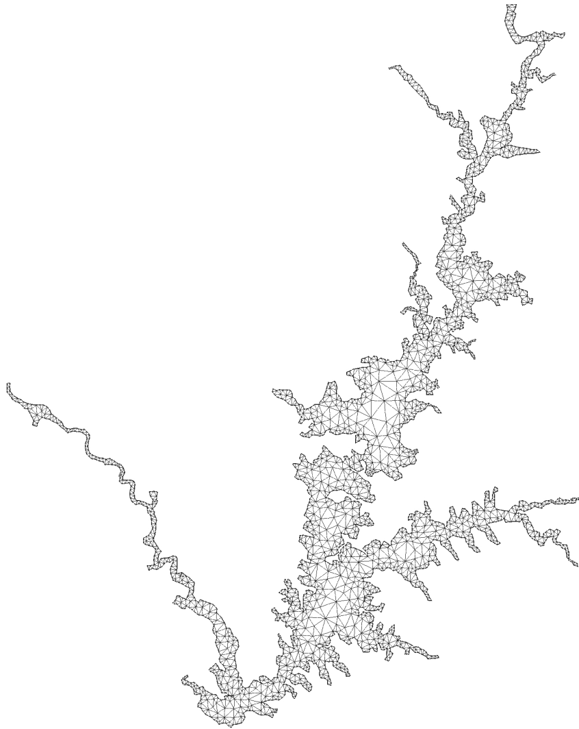
Figure 5.3 - Detail of medium definition mesh M2 for Alqueva showing southern area. Distance between nodes: 1174 m (Maxima); 338 m (Average).
