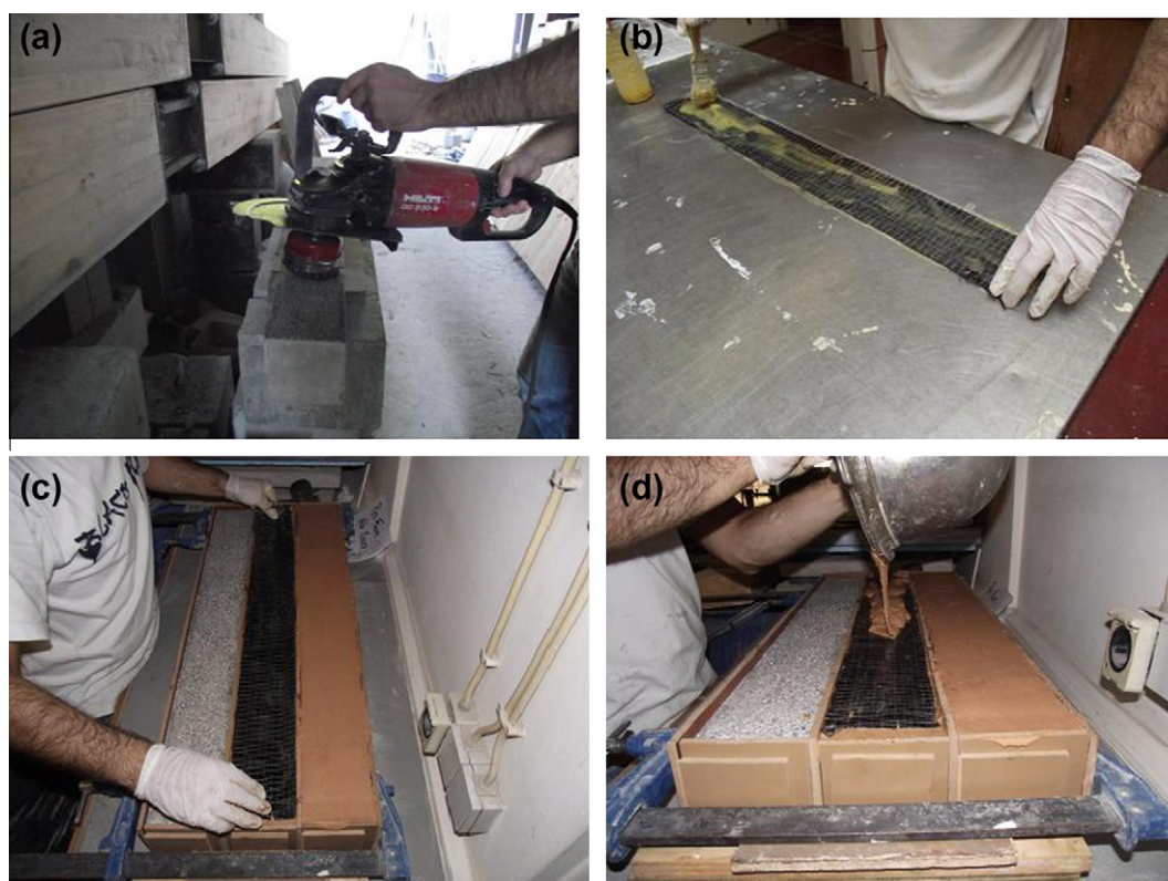
Fig. 5. OPC concrete beams preparation: (a) surface roughening; (b) CFRP sheets impregnation; (c) Placing the CFRP sheet over the geopolymeric mortar; (d) applying a second layer of geopolymeric mortar.
