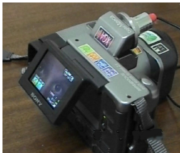
Fig. 2. The portable photorefractor showing the acquired image used for illustrating the processing process (Figs. 3–5).
