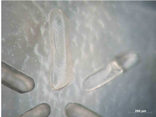
Figure 6.35. Detail view of the high-relief UM logo on PP (10×)
