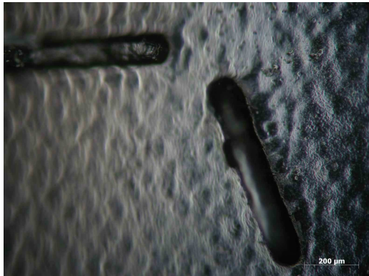
Figure 6.55. Microscopy image of a low-relief microdetail on the POM plastic part
