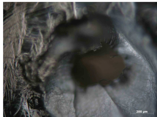
Figure 6.42. Detail view of Pin 2 moulded with POM on the BA01SLM block (10×)
