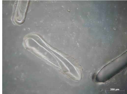
Figure 6.36. Detail view of the high-relief SE logo on PP (10×)
