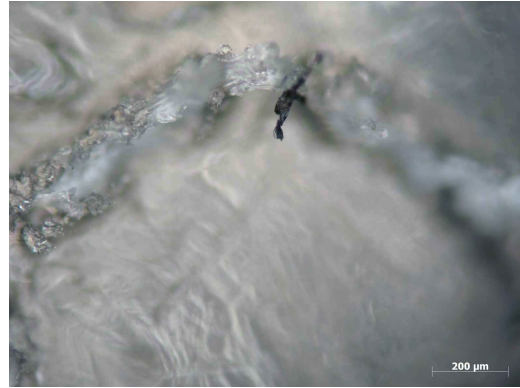
Figure 6.47. Top view of the high-relief UM logo on PP (10×)
