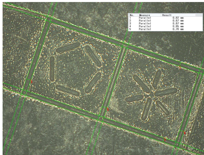
Figure 5.15. Sample of hybrid microscopy measurements obtained with the Keyence VHX-500F
