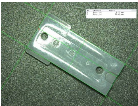
Figure 6.6. BA01SLA moulding block, top side (magnified 10×)
