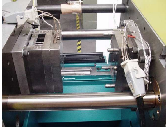
Figure 4.21. Micromould showing electrical and sensor connections
