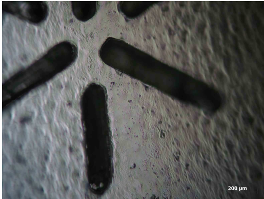
Figure 6.31. Detail view of the low-relief UM logo on POM (10×)
