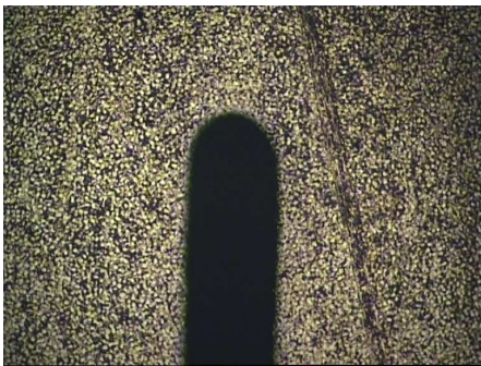
Figure 6.8. Rib detail on the MS01 moulding block manufactured by microEDM
