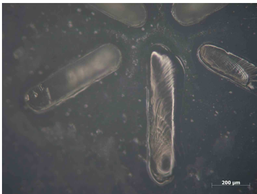
Figure 6.77. Top view of high-relief SE logo at the low-relief area of the part (10 \times )
