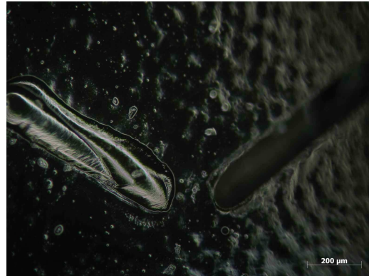
Figure 6.32. Detail view of the low-relief SE logo on POM (10×)
