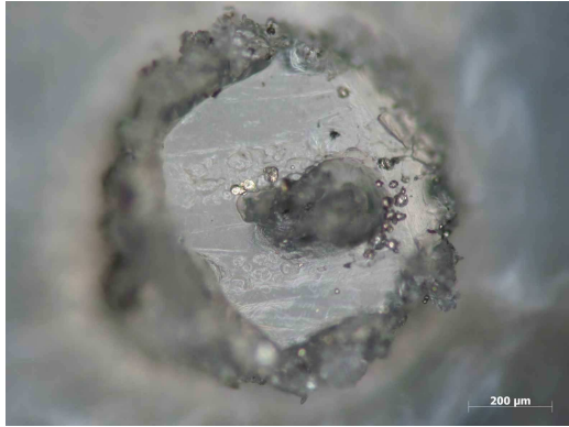
Figure 6.42. Detail view of Pin 1 with PP on the BA01SLM block (10×)
