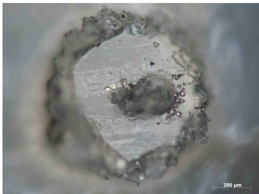
Figure 6.58. Microscopy image of Pin 1 moulded with PP
