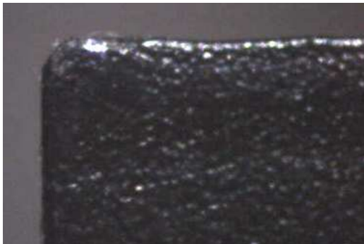
Figure 6.50. Replication of microEDM surface on to the rib of MS01 moulding block with POM
