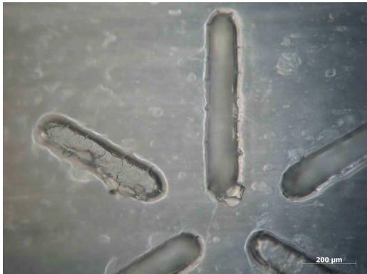
Figure 6.37. Detail view of the low-relief UM logo on PP (10×)
