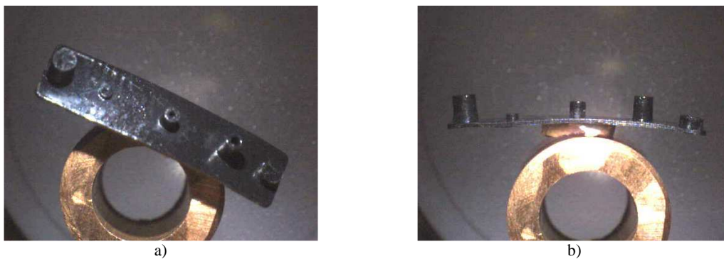
Figure 6.27. Plastic parts obtained from the BA01SLA block
