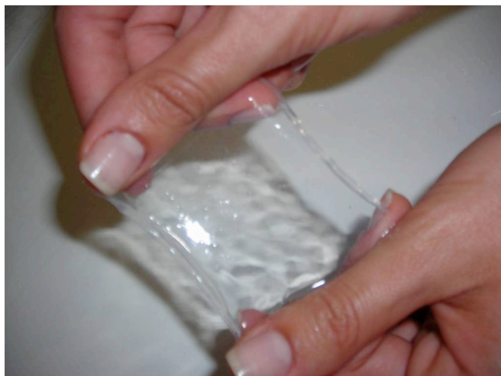
Figure 8. Bacterial cellulose pellicle produced by ATCC 10245 G. xylinus strain in static culture.
