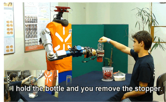
Fig. 1. The anthropomorphic robot acts as a pro-active personal assistant of a person, with motor impairments, that wishes to drink.
