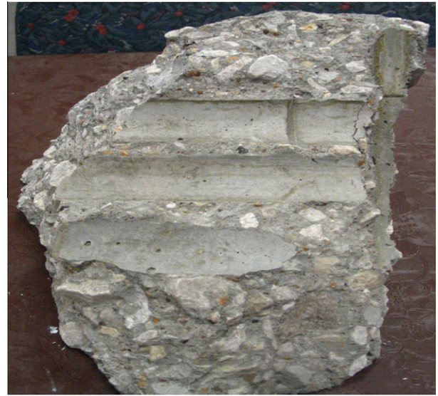
Fig. 5. Imprints of bamboo reinforcement [46].
