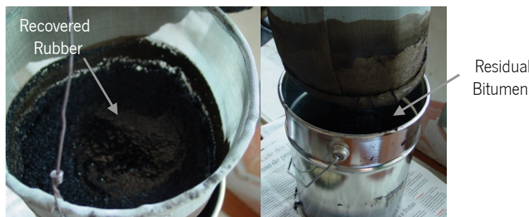
Figure 5.6 – Appearance of the residual bitumen and recovered rubber from the AR binder
