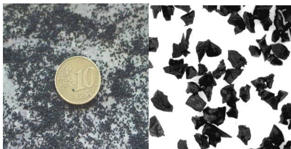
Figure 5.90 – Macroscopic and microscopic appearance of the crumb rubber particles
