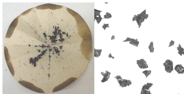
Figure 5.93 – Macroscopic and microscopic appearance of the rubber particles recovered from the AR produced with the base bitumen I
