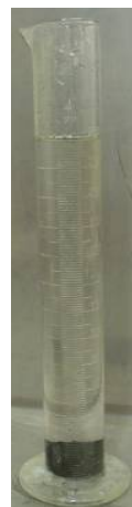
Figure 5.89 – Appearance of the crumb rubber in water at 25 \text{ }^\circ\text{C} after application of standard test AG:PT/T144
