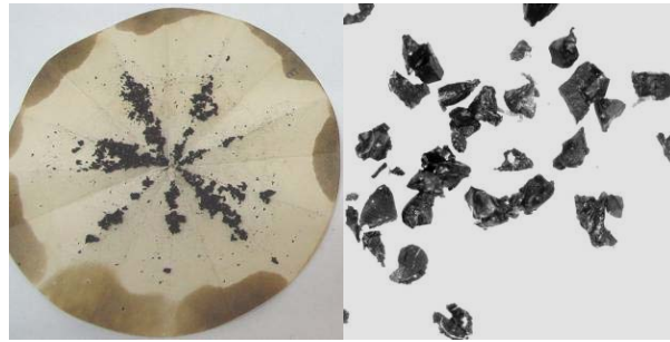
Figure 5.92 – Macroscopic and microscopic appearance of the rubber particles recovered from the AR produced with the base bitumen E
