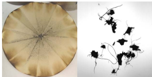
Figure 5.98 – Macroscopic and microscopic appearance of the rubber particles filtered from the residual bitumen of the AR produced with the base bitumen M
