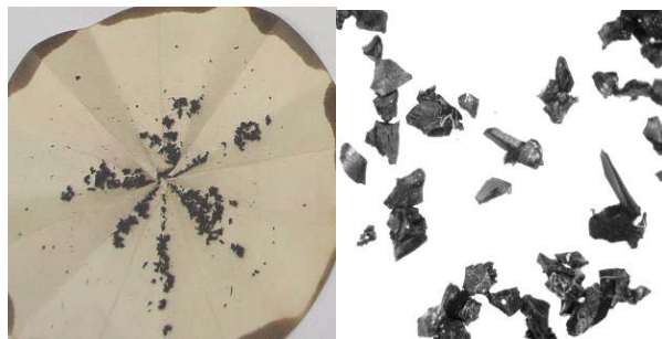
Figure 5.91 – Macroscopic and microscopic appearance of the rubber particles recovered from the AR produced with the base bitumen A
