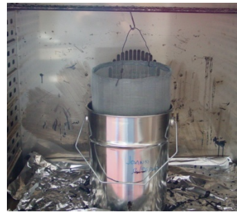
Figure 5.5 – Separation of the crumb rubber and residual bitumen from the AR binder
