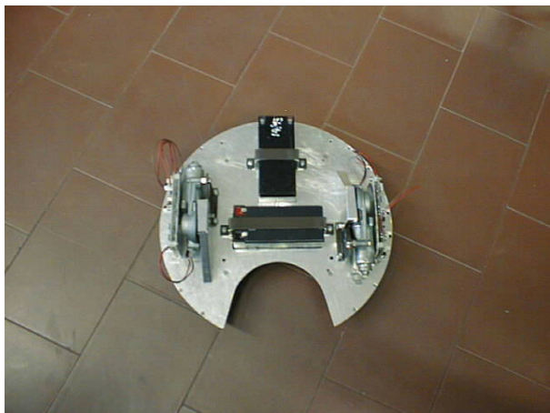
Fig. 4. "Prometeu" robot base where motors, wheels and batteries are placed.
