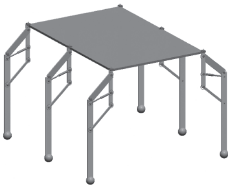
Figure 2 · Mechanical structure of the hexapod robot.
