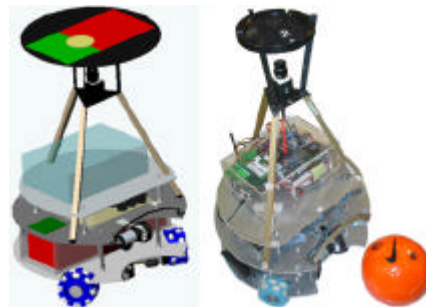
Fig. 2. CAD drawing of the complete robot and final real robot
