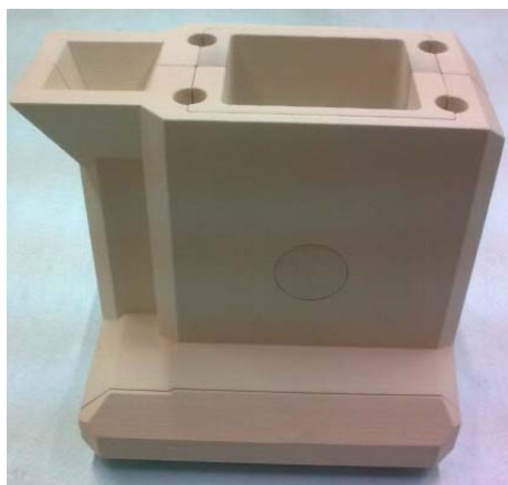
Figure 12. Fully assembled mould ready for metal pouring
