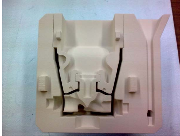
Figure 11. Half assembled mould showing coolant chamber and top chamber cores, the pouring basin, the sprue and the runner entrance
