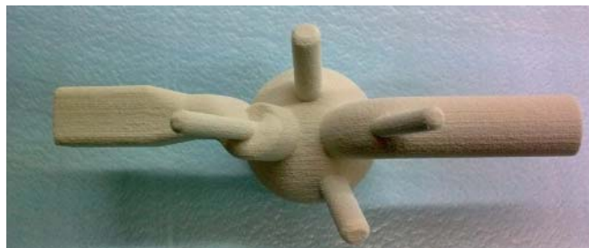
Figure 10. Combustion chamber, inlet and exhaust passages inner core (note the swirl geometry)
