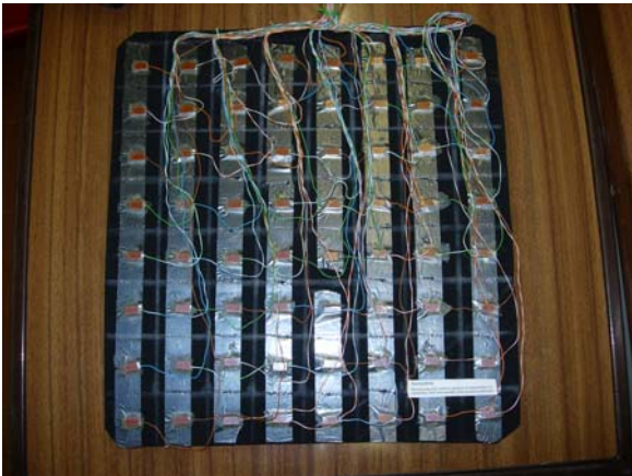
Fig. 6. Picture of the sensor array before its placement inside the cushion.
