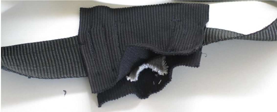
Figure 4. Accessory using knitted fabric as extension sensor.
