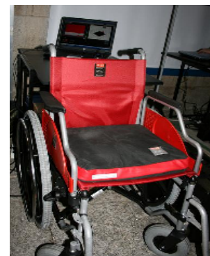
Fig. 11 - First cushion prototype equipped with the sensor matrix and the monitoring system.
