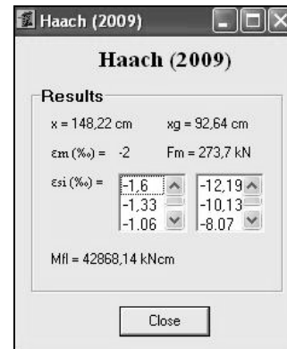
Figure 7.33 – Results of software RMW for the flexural design of wall P16 at the basement.
