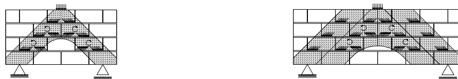
Figure 6.44 – The way of stresses from the point of application to the supports through the bed joints.
