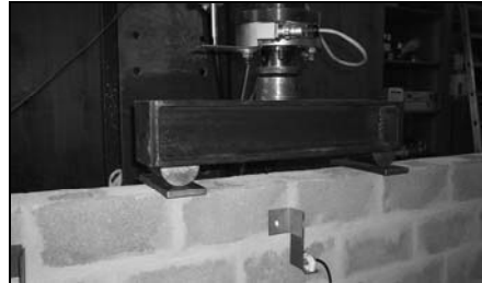
Figure 5.6 – Load configuration for the four point load bending test
