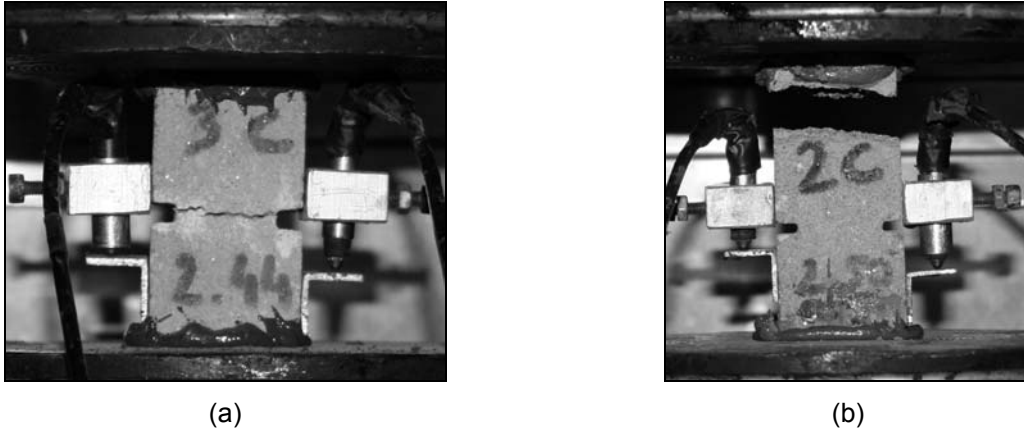
Figure 3.6 – Fracture of the specimens in direct tensile test: (a) common fracture and (b) fracture in zone with higher cross section.
