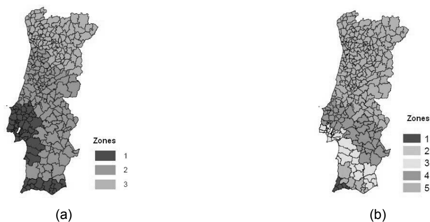
Figure 7.27 – Zoning for seismic action with a return period of 475 years: (a) near action and (b) distant action.
