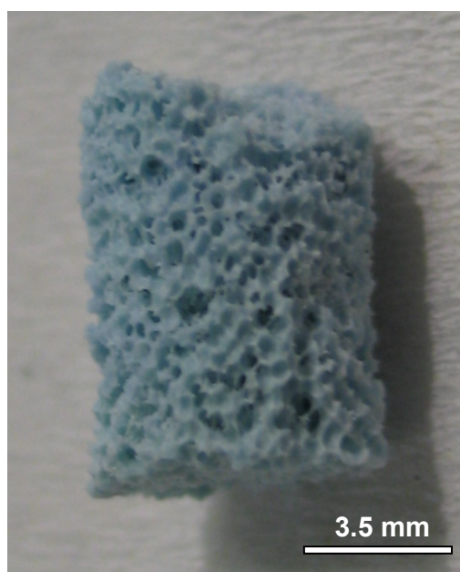
Figure 2. Macroscopic appearance of the HAp scaffolds after sintering at 1300°C.
