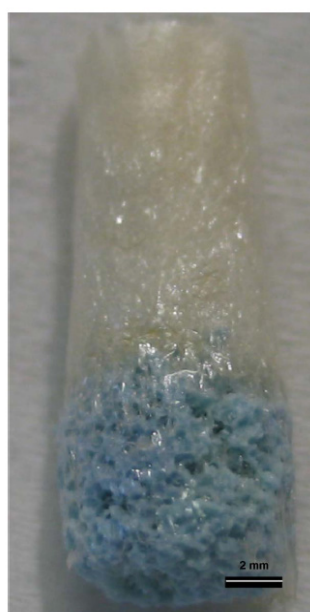
Figure 1. Macroscopic appearance of the HAp/CHT bilayered scaffolds.
