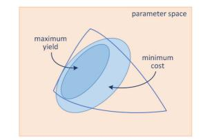
**FIGURE 4.** Two regions of design parameter values statistically generated around a maximum yield design and a minimum cost design, respectively; the region of acceptable designs is enclosed by the thin curved lines [40]. The corresponding nominal designs could be anywhere within those regions, depending on the constraints, tolerances, and probability distribution function of each individual design variable.
