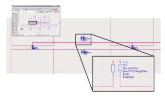
FIGURE 16. Tuning ports: Example using Agilent ADS to tune coupling between resonators. Most of the filter is EM analyzed in Sonnet. Tuning is done in ADS [159]. Courtesy of Jim Rautio.
