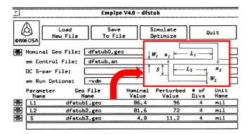
**FIGURE 8.** A 1996 Empipe<sup>TM</sup> Geometry Capture user interface setup for direct electromagnetic optimization of a double folded stub microstrip filter in Sonnet Software's *em*<sup>TM</sup> [69].
