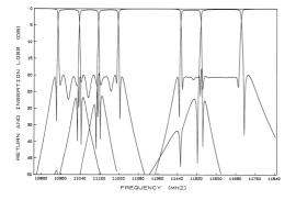
**FIGURE 6.** Optimized 5-channel noncontiguous waveguide multiplexer using 75 optimization variables. From [55].
