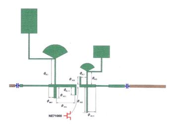
**FIGURE 13.** Circuit structure of a class B frequency doubler with ten geometrical optimization variables [105]. The circuit is derived from a Microwave Engineering Europe challenge [104].
