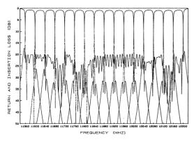
FIGURE 5. Optimized 16-channel waveguide multiplexer using 240 optimization variables. From [11].
