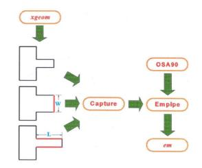
FIGURE 12. Example of Geometry Capture for parameterizing a microstrip step structure. From [105].
