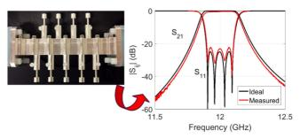
FIGURE 18. Space mapping applied to physically tune, in a few "iterations," a 4-pole inductively coupled rectangular waveguide filter with tuning screws in cavities and coupling windows [186]. Courtesy of Vicente Boria and Marco Guglielmi.
