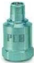
*Industrial ceramic shear ICP® accel., 100 mV/g, 0.5 to 5000 Hz, 2-pin top connector*
