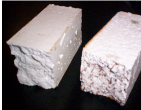
Fig. 1 – Gypsum plasters with cellulose fibres and cork
