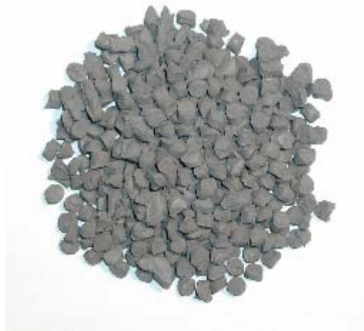
Figure 2.4 An example of PIM feedstock in pellet form, ready to feed into the injection moulding machine.
