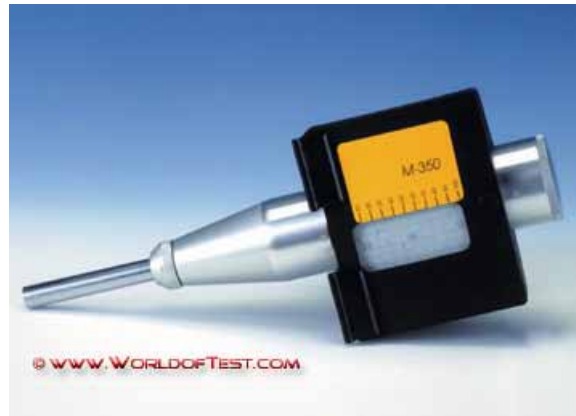
Fig. 4-24 Rebound Hammer, Manual Model W-M-350 produced by Qualitest company
