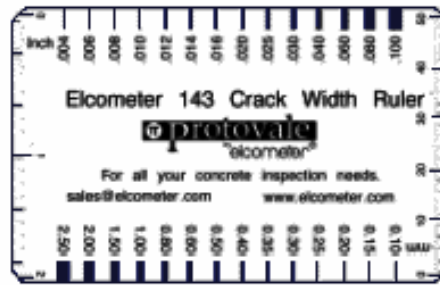
Fig. 4-21 Crack width ruler produced by Elcometer
