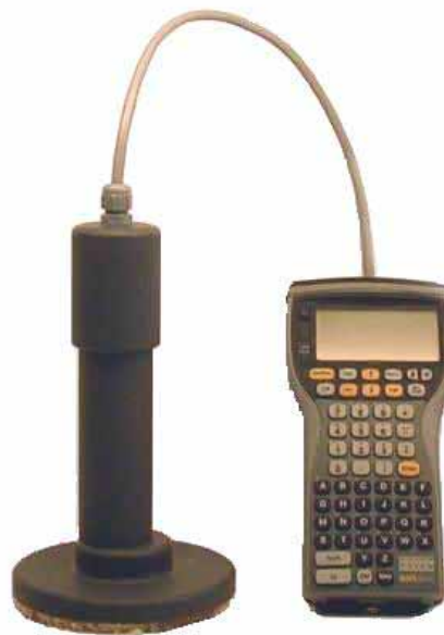
Fig. 4-13 Galva Pulse instrument manufactured by Germann Instruments
