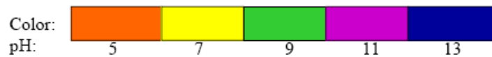
Fig. 4-18 Rainbow Test – colours of sprayed concrete against its pH value (German Instruments 2003)
