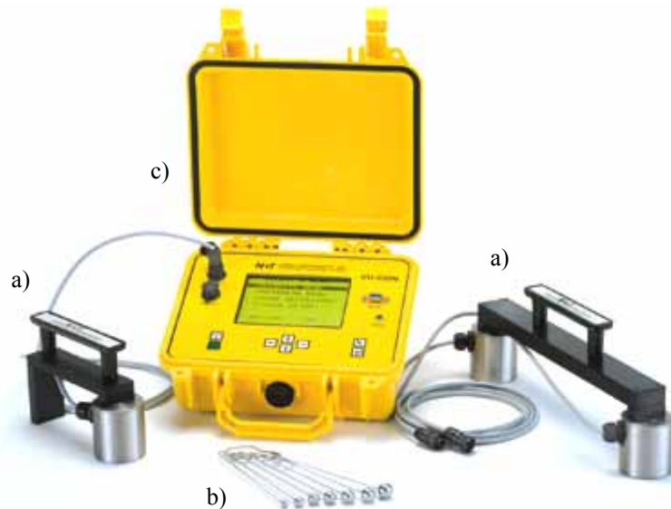
Fig. 4-3 Impact-Echo Test System provided by James Instruments Inc.
