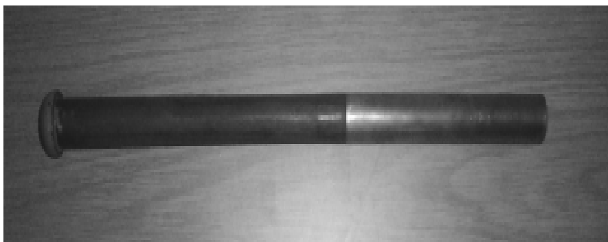
Figure 3. Two-piece rod made of iron and nylon
