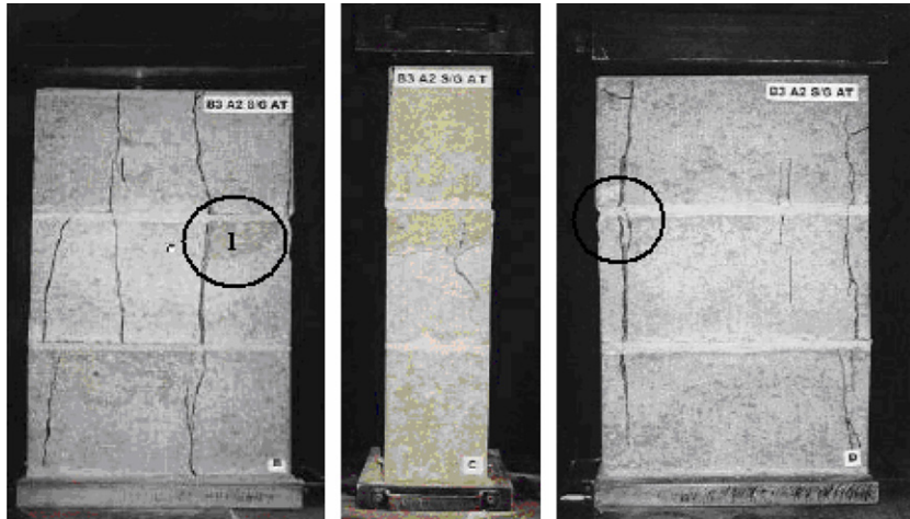
Fig. 15. Observed failure modes for hollow concrete block prisms [17].
