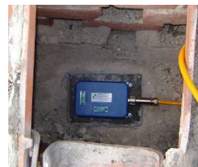
Figure 9. Dynamic monitoring system: (a) location of the accelerometers (A1 on the base and A2 on the top of the vault nave); (b) sensor A2 directly on the vault extrados; (c) strong motion recorder (analyzer)
