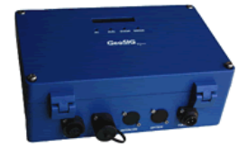
Figure 9. Dynamic monitoring system: (a) location of the accelerometers (A1 on the base and A2 on the top of the vault nave); (b) sensor A2 directly on the vault extrados; (c) strong motion recorder (analyzer)
