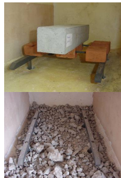
Fig. 4 – Before and after test: explosive spalling
